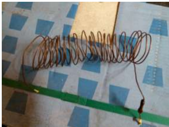
Fig. 3 Capillary Tube 1 Size: d= 0.031 -inch, L= 11 feet
