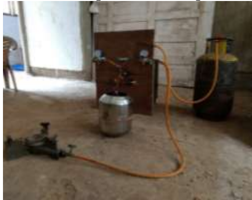
Fig. 1. Basic experimental setup of LPG refrigeration system
